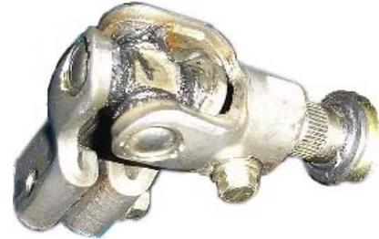
Another common failure we see is adhesive failure of a shaft and coupler which has been bonded together with some sort of 'super dooper epoxy'. Your steering system is no place for bonded joints. The better way to couple any of your steering components together is with splined joints.
