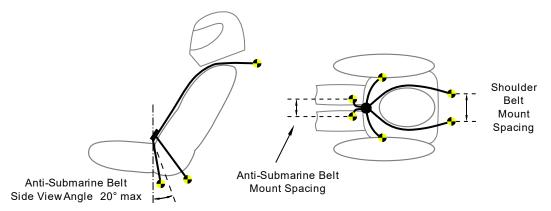
b. With the Anti-Submarine Belt Mounting Points on the Primary Structure at or near the Lap Belt anchorages, the driver sitting on the Anti-Submarine Belts, and the belts coming up around the groin to the release buckle.
