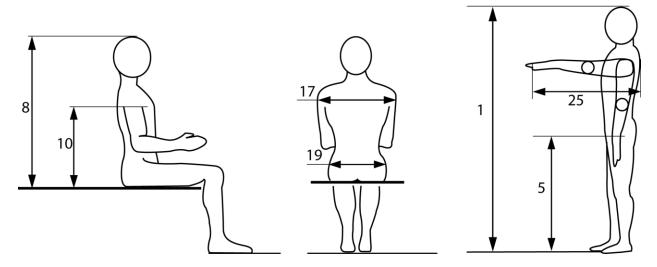
In designing your car for this range of builds, you do not have to have the same seat or seat insert for all drivers. The idea is that the one basic car design should be able to accommodate, and hence be saleable to, drivers of a range of statures from the 5th percentile female to the 95th percentile male.
