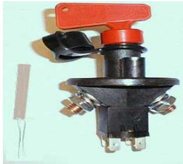
IC4.2.2 The master switches must be mounted so that the rotary axis of the key is near horizontal and across the car. The “ON” position of the switch must be in the horizontal position and must be marked accordingly. The “OFF” position of the primary master switch must also be clearly marked.
