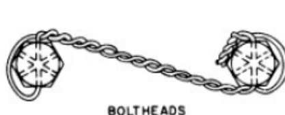
FIGURE #31 – SAFETY WIRED BOLT PAIR- SOURCE MS33540
