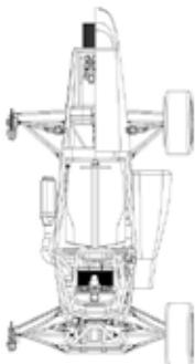
**BRAKE :** All wheel Brembo P34C brake calipers/cross drilled mild steel floating rotors
