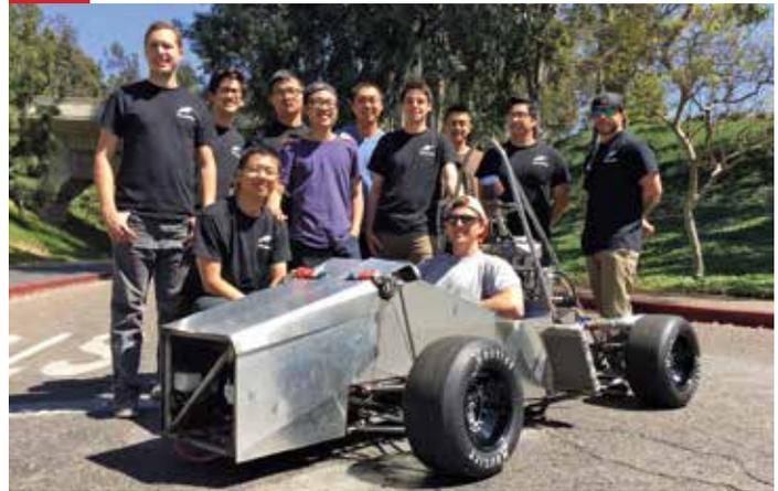
Meet "Savage", the successor of UC Irvine's 2015 racecar, AR-9. Learning from last year's failures, Savage has gained strength in it's brethren's pitfalls and lost weight. A complete aluminum steering assembly, composite seat, data logger, and reduced un-sprung mass have been incorporated while packaging all around the vehicle has been improved. Meanwhile, Savage has revamped yet maintained it's unique WWII-era styling cues with a 3003 aluminum body.
