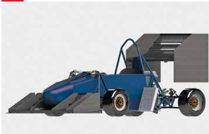
This year's car UTR-22, was built around simplicity and reliability while also taking on some new features. Utilizing tire consortium data as a starting point, UTR-22 features a rigid tubular chassis, CBR600 F4i, and Ohlins shocks backed up with extensive durability testing. Serviceability and weight reduction were also considered with every component designed. With a large amount of time dedicated to testing and refining we hope to have an all-around reliable and fine-tuned car for competition.
