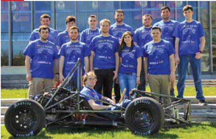
The 2016 car includes mild improvements over the previous Corsair Racing car. A new engine, provided by a 2006 Suzuki GSX-R 600, is mated to a solid rear axle through a 45-tooth sprocket. Redundant frame bracing has been removed to lighten the structure, and an angle has been added to the front structure to prevent scraping under heavy braking.
