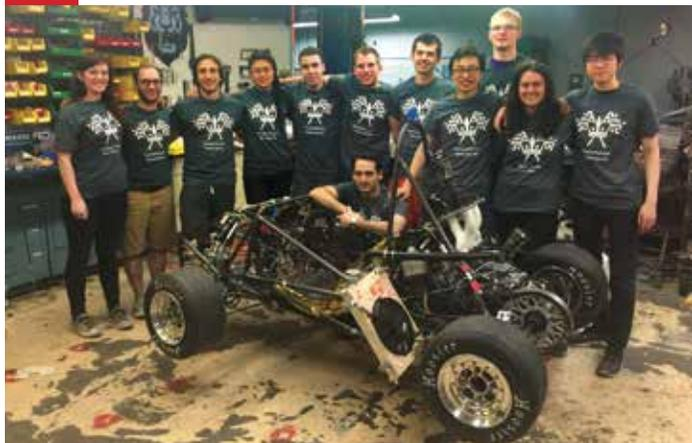
Knickerbocker Motorsports is introducing an entirely new platform, KMR-16, outfitted with 10" tires to reduce moment of inertia, a CBR600RR engine for optimal power, and an electro-pneumatic shift-clutch mechanism.
