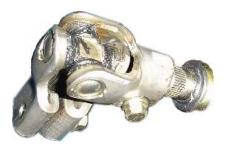
Another common failure we see is adhesive failure of a shaft and coupler which has been bonded together with some sort of 'super dooper epoxy'. Your steering system is no place for bonded joints. The better way to couple any of your steering components together is with splined joints.
